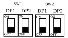
The 2 dipswitches in SW1 adjust the charging curve as shown in the table below.
